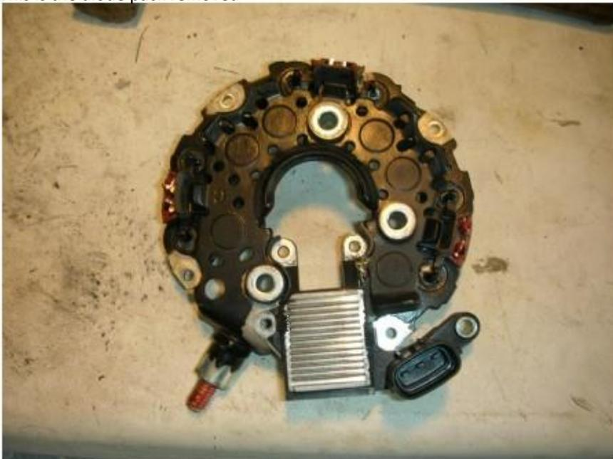
You now need to remove the silver vaned rectifier by removing the solder from the connection from the copper tag, this needs to be re-soldered on to the new diode pack.
