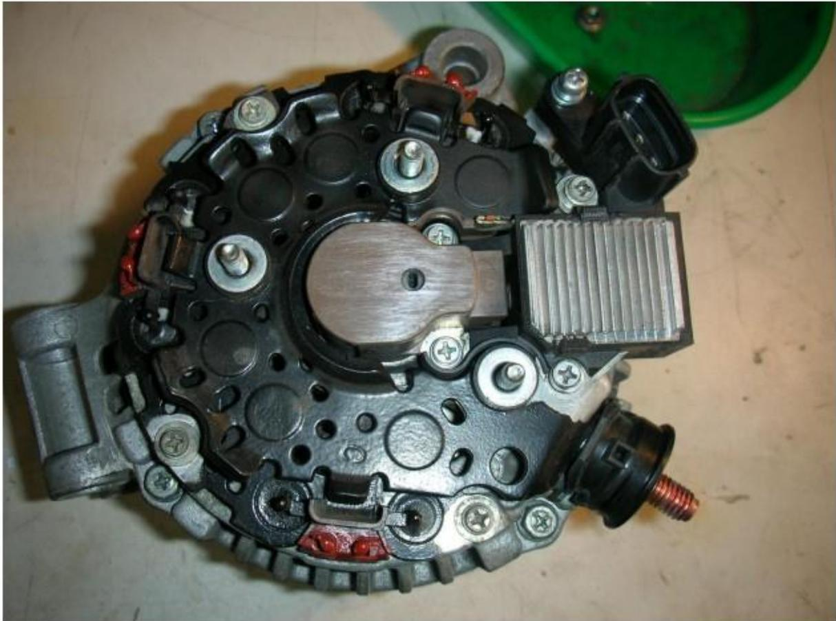
Now remove the two screws holding the brown carbon brush holder in the centre of the unit, then just lift it off and put it somewhere safe out of the way.
