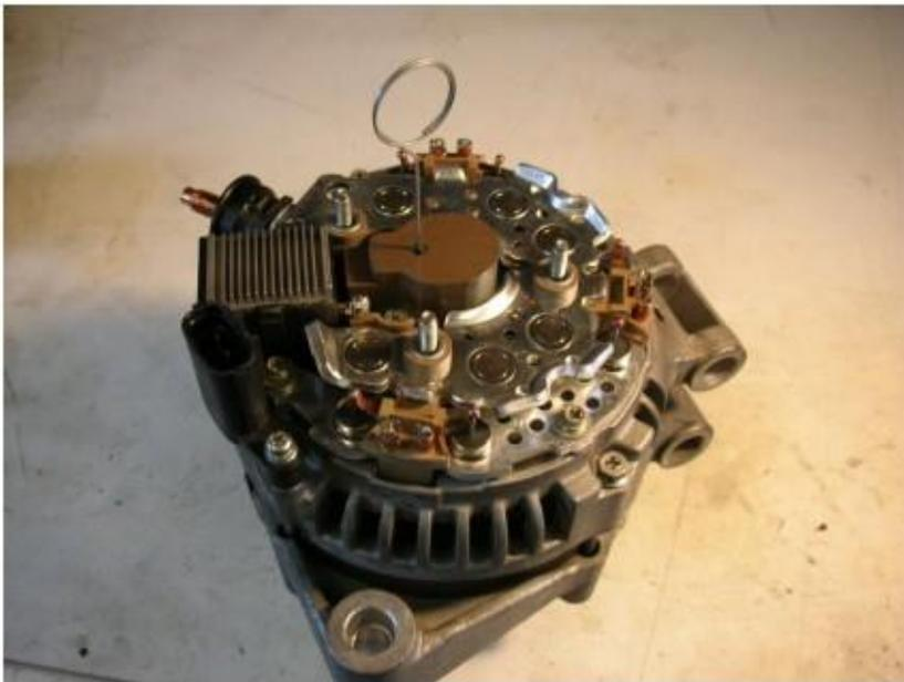
Slide the holder back on to the main shaft and secure using the two screws then once all secure pull out the pin and you should here the brushes click against the main shaft.
