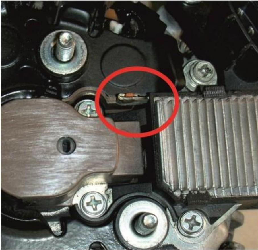
As you can see in the picture below there are two diodes that have blown apart there was a total of 5 that were in this condition.
