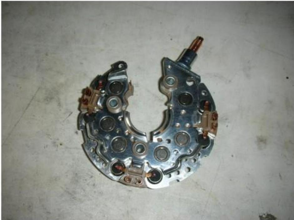
Slide the new diode pack over the three studs making sure the six copper wires come through in to the three connectors that you will now re-solder back on to the diode base plate.
