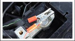
Connect black crocodile clip to **negative** battery lead (**black** cables going to it, towards **REAR** of battery box on D3/D4/RRS)
