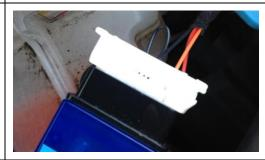
Remove battery cover and connect red crocodile clip to **positive** battery lead (**red** cables going to it, towards **FRONT** of battery box on D3/D4/RRS)
